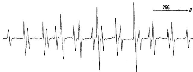
FIGURE 2 E.s.r. spectrum of TEMPO with \text{GaCl}_3 under conditions where only species (II) is present
